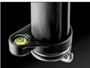
Adjust the inclination of the centre column to get it perfectly level, using the built-in bubble spirit level as a reference. Once correctly leveled and locked, the centre column can be extended to the required height without affecting inclination.
