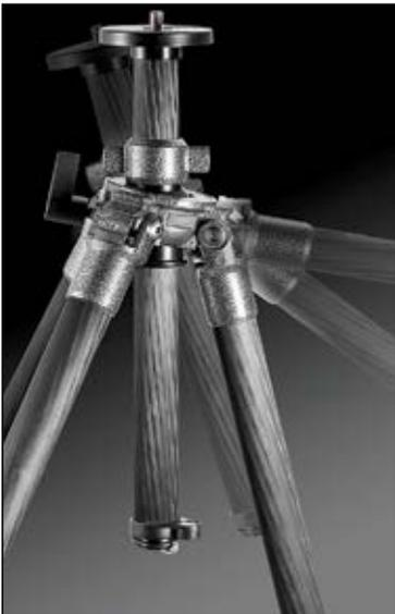
The centre column can be inclined in any direction at any angle up to 15°. Leg angles can be set independently at any of the three positions. A leveling tripod is an ideal support for fluid heads, setting the camera perfectly horizontal while allowing the fluid head to control pan and tilt movements.
