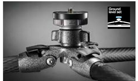
The Ground Level Set mechanism, which lets the photographer remove the centre column to get the camera closer to the ground, has been completely redesigned for faster operation. A single simple unlocking ring under the column's upper disc frees the column while keeping the upper disc solidly in place on the tripod, with no need to unscrew and re-fit the upper disc and hook as in previous versions.
